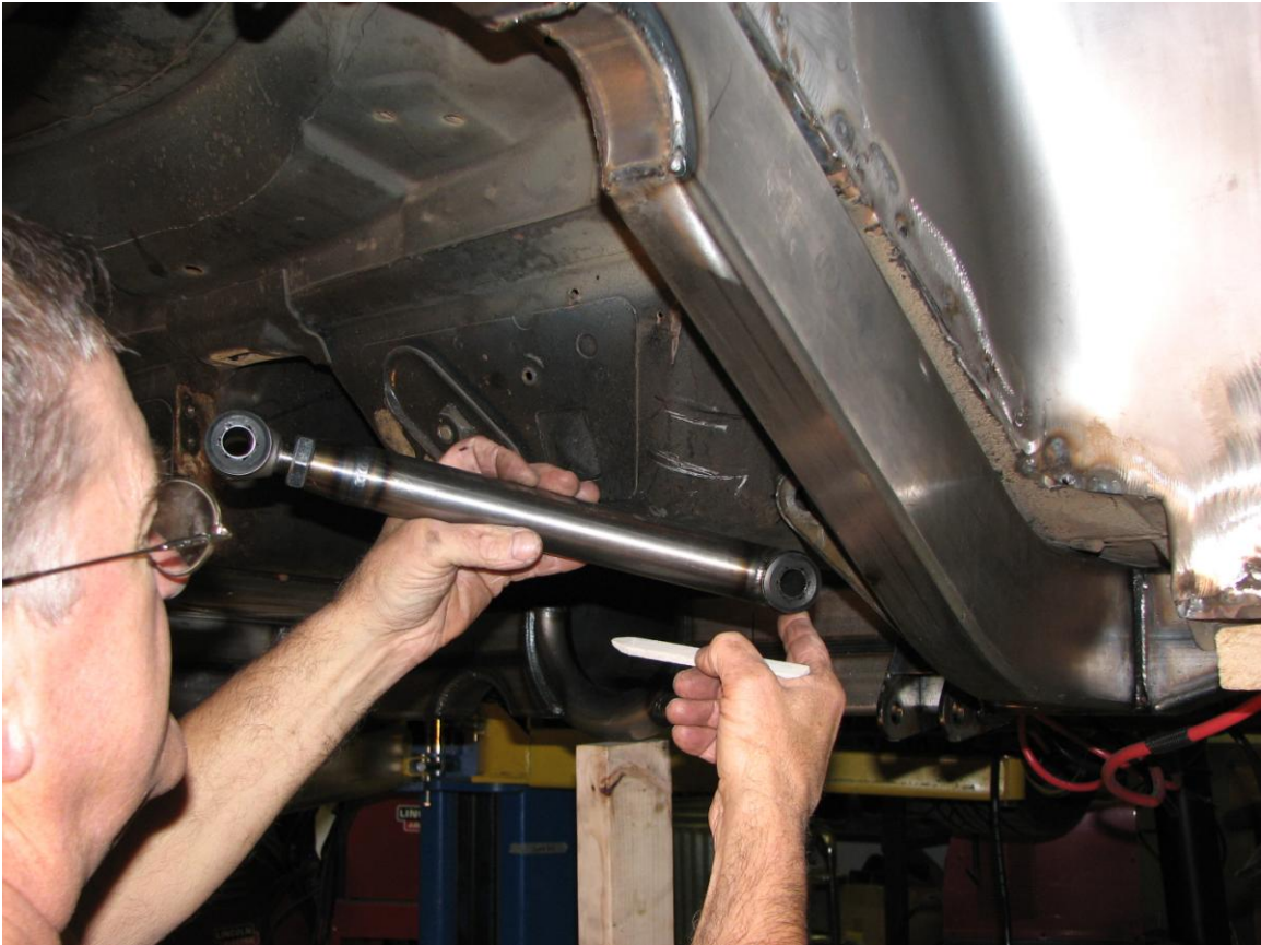
(Photo 5) UCA Tube Clearance: If more clearance is needed, use a section of 1.5" or 2" tube to dent the area. Simply rotate the link until contact is made, then draw an outline of the tube to serve as a guide.
