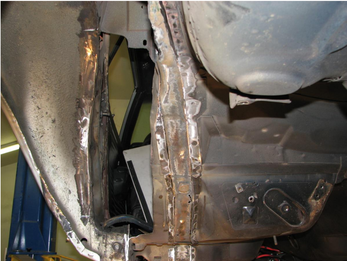
(Photo 2) Rail has been fully removed, but the spot-welded strips remain on the vehicle to save time. They may be removed if desired. This vehicle has had the factory inner wheeltubs removed at the same time in preparation to install Detroit Speed's wheeltubs.
