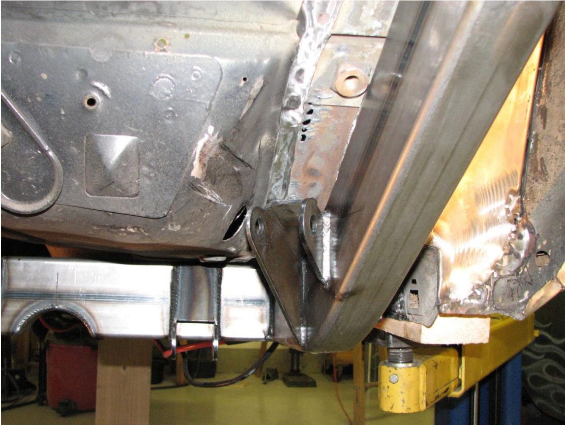
(Photo 3) Access Holes: On triangulated 4-bar suspensions, 1.5" holes need to be drilled to gain access to the upper control arm bolt. Use the provided plastic plugs to seal the hole after the suspension has been installed.
