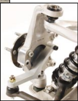
Morrison has re-engineered the C6 front spindle with a lower steering arm mount. This allows the rack to be mounted 2" lower in the chassis, providing extra engine clearance and a lower center of gravity!
