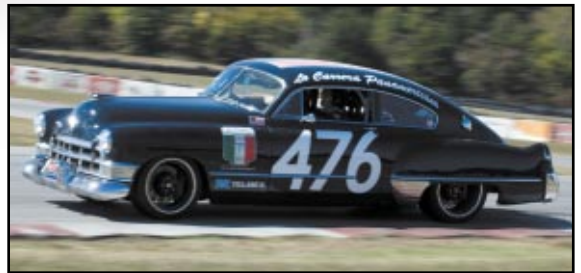
Hayden Groendyke used a custom AME Max-G chassis under his 1949 Cadillac to compete in the 2010 La Carrera Panamericana road race.
